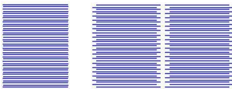
Fig.2-196 Left is the expectation of processing, the right is processing effect of transmission lag
